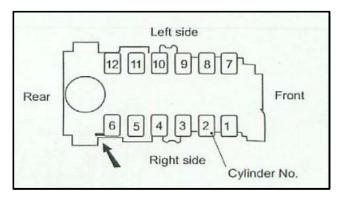
the S16R engine serial number is stamped on the nameplate and is located at the left front side of the engine.
