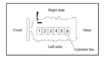
the S12R engine serial number is stamped on the nameplate and is located at the left front side of the engine.
