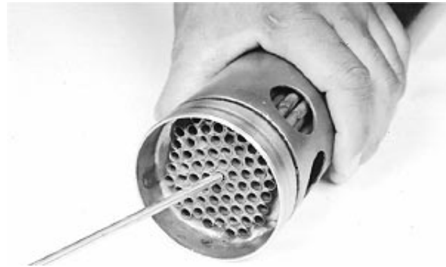
Clean Heat Exchanger
